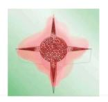
The pink area is stressed, which improves hole stabilization and increases the drilling window.
